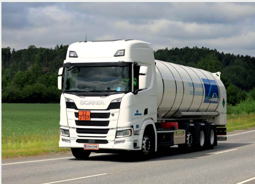
Cryogenic liquid \text{CO}_2 distribution by road
