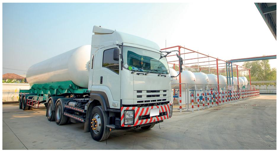
testing, and maintenance also transfers. The periodic inspection requirements are country-specific, but a hydraulic test and visual inspection every 10 years is typical.
