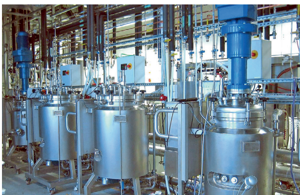
Figure 6. A pilot plant in Munich undertaking the biotechnological process of anaerobic digestion to create biofuel.
