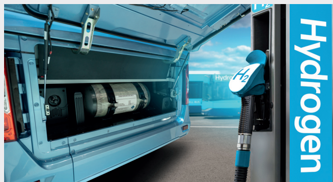
Compressed hydrogen gas storage in a bus
