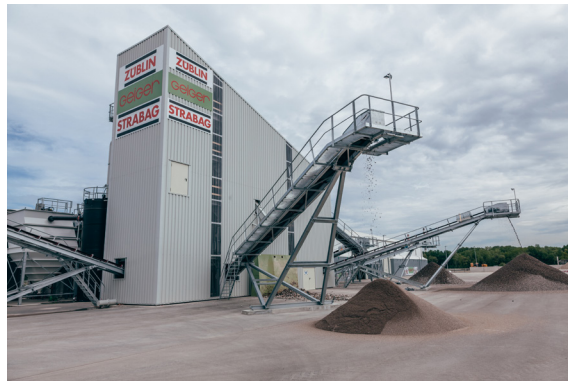
Copyright ZÜBLIN Umwelttechnik GmbH, In-situ soil washing and grading process unit
