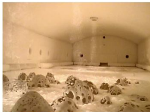
COROX® convective glass melting in operation
