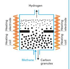
Moving Carbon Bed Methane Pyrolysis
