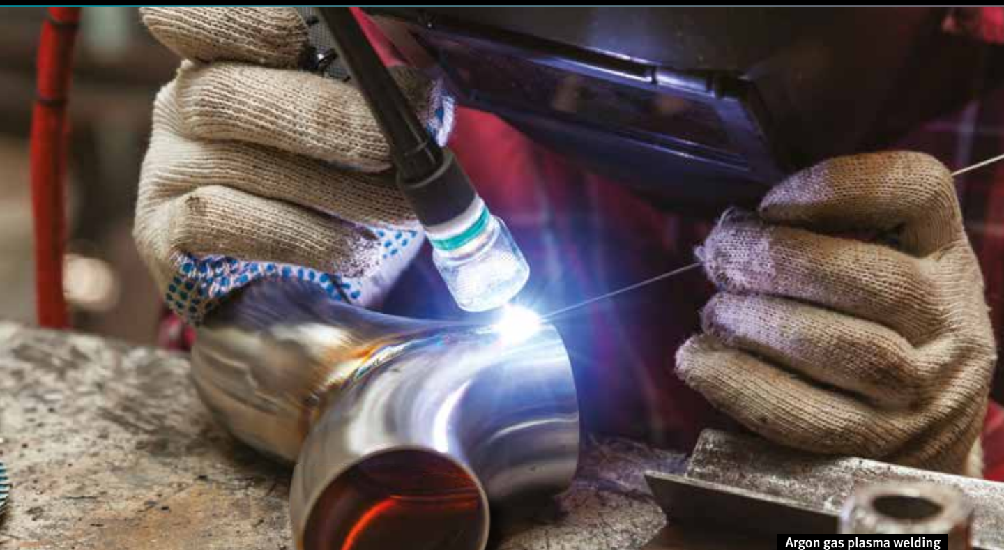
Argon gas plasma welding
